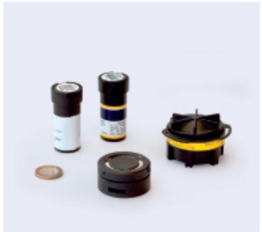
*Measuring devices for determining the radon concentration*
