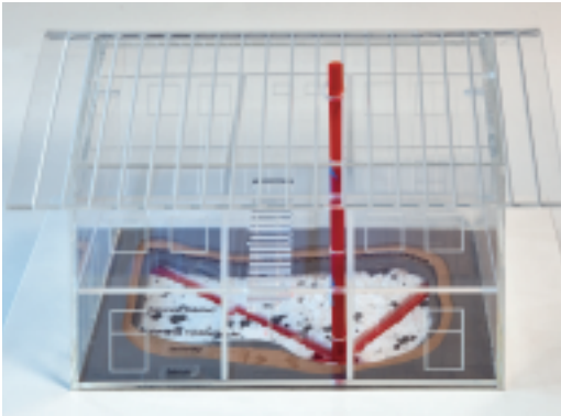
Model: Sub-floor suction, vented through the roof (full-wall pipe with a diameter of at least 15 cm)
