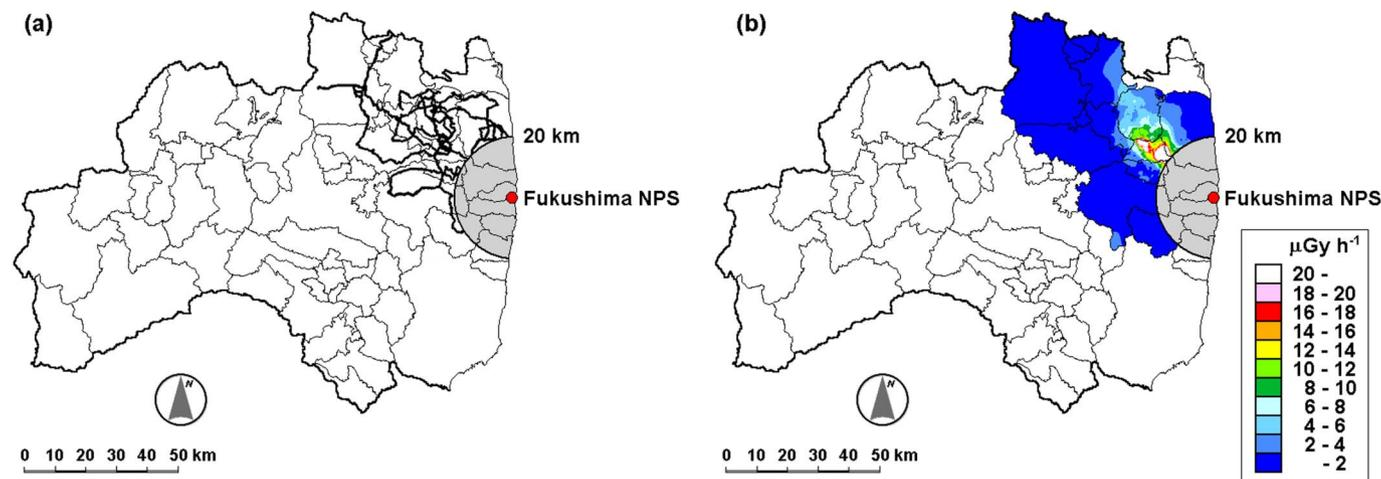
**Figure 3** | (a) Survey route for measuring dose rates in air within the high level contamination area. Total distance for the car-borne survey in this area was 730 km. (b) Distribution map of the dose rates in air within the high level contamination area in Fukushima Prefecture. The rates were classified into eleven groups from  $<2 \mu\text{Gy h}^{-1}$  to  $>20 \mu\text{Gy h}^{-1}$  at intervals of  $2 \mu\text{Gy h}^{-1}$ .
