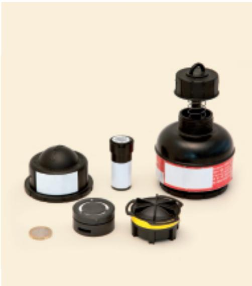
*Devices used to measure the radon concentration*
